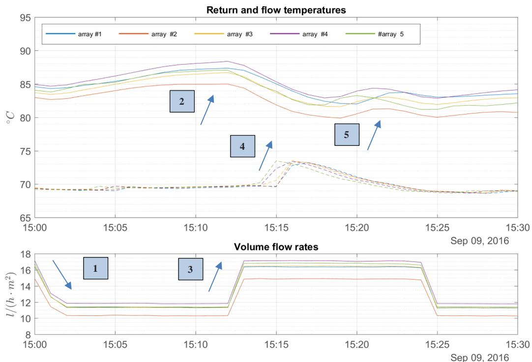
**Fig. 5: Delayed response of the collector array outlet temperature (2, 5), when swift changes of the volume flow rate (1, 3) and return temperature (4) occur. Depicted are five arrays of the test plant.**
