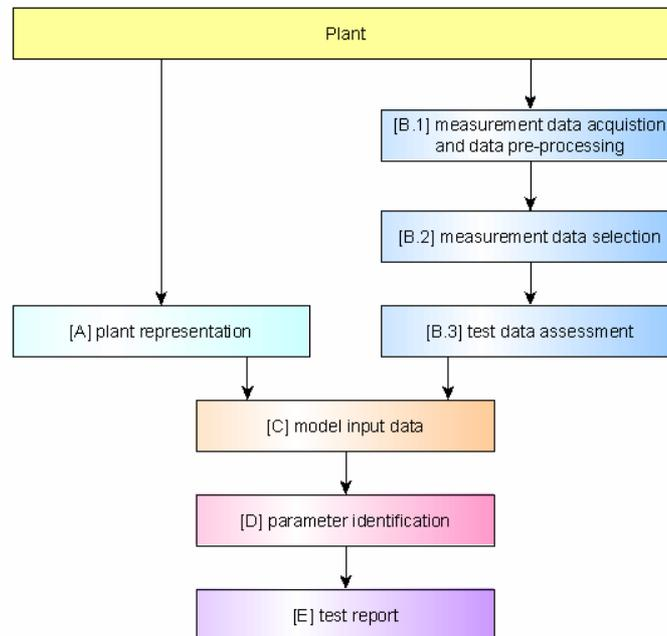
Fig. 1: Flowchart of the in-situ collector array test
