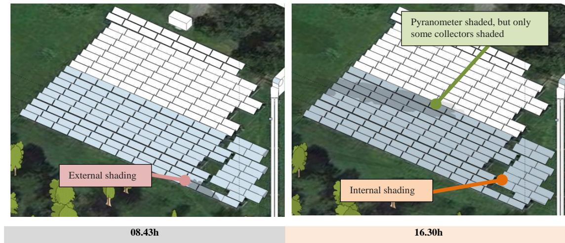
Fig. 4: Irradiance analysis of the test plant (2017-09-27)
