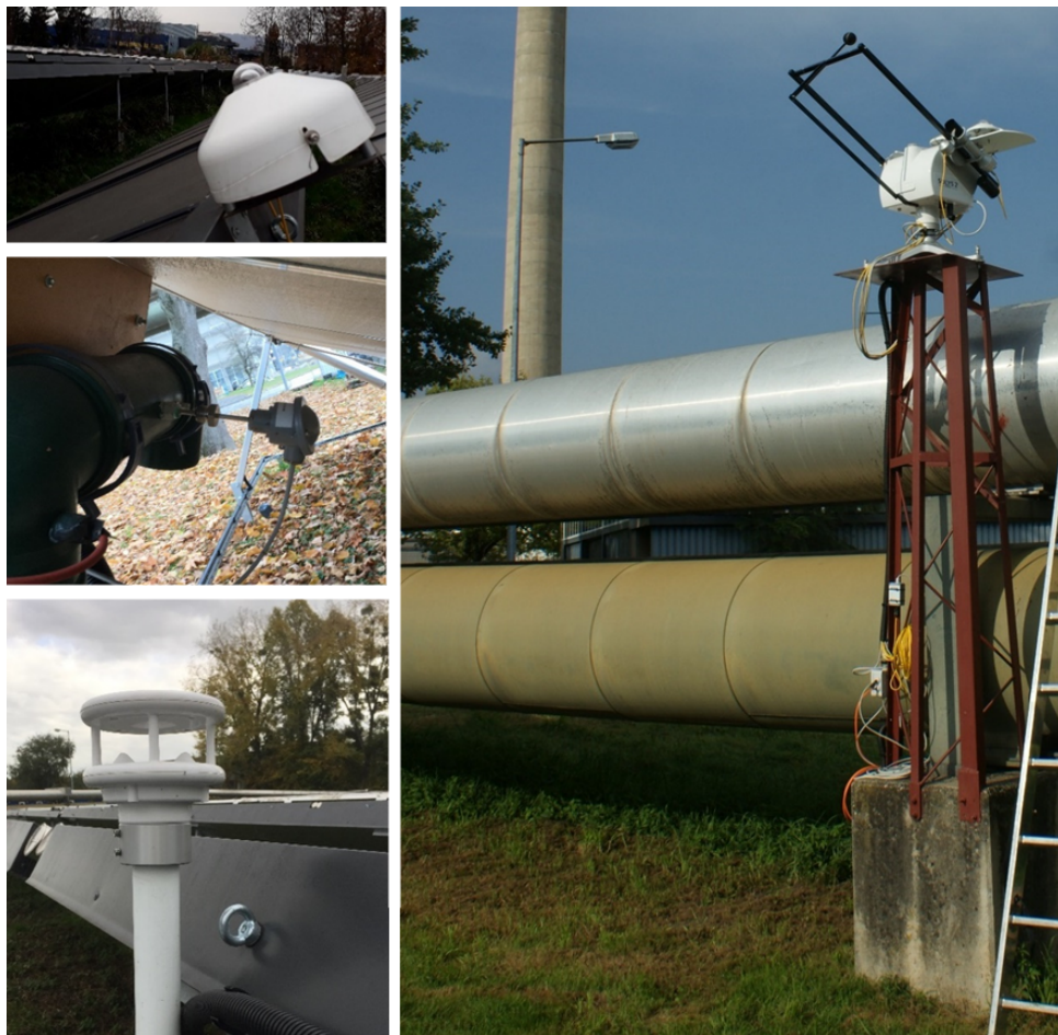
Figure 11: Pyranometer (top left), ambient temperature sensor with ventilation unit (middle left), wind sensor (bottom left) and radiation platform including pyrheliometer and unshaded and shaded pyranometer (right).
