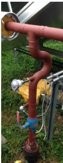
Figure 10: Temperature measurement at the mixed outlet of all rows of one collector array (left). Temperature measurement between collectors (right).
